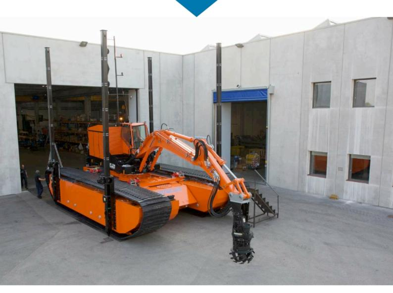
DRM85/180 (Multi-Purpose series) represents a step over on approach of dredging technique. The extreme mobility in any kind of swamp, together with the full floatability, allow to reach the most remote locations otherwise impossible to get with any other equipment.
